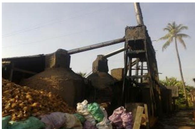
FIGURE 11: CHARCOAL MAKING KILN FROM COCONUT SHELL
